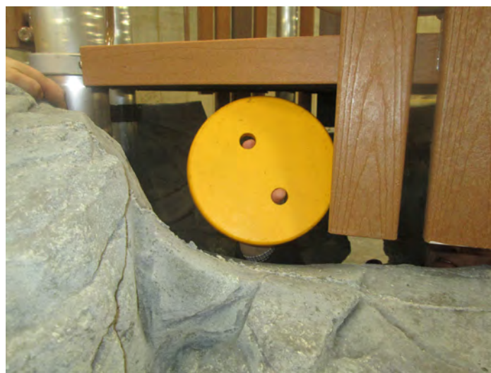
INSPECTION C Place head template between deck and rock. Template should be perpendicular to the opening. Head template shall pass between deck and rock.
