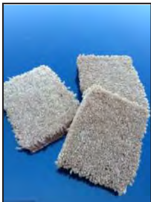
PADDING FOR PROTECTION. ONLY NEEDED IF USING LIFTING STRAPS
